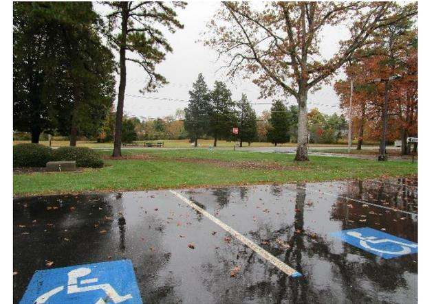
Parking spaces can be converted to porous pavement to capture and infiltrate stormwater runoff from the parking lot. Rain gardens can be installed in the turfgrass area on the eastern corner to capture, treat, and infiltrate stormwater runoff from the lot and in front of the building to capture rooftop runoff. A preliminary soil assessment suggests that more soil testing would be required before determining the soil's suitability for green infrastructure.
