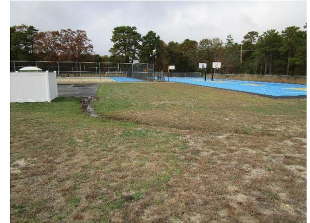
A rain garden can be installed in the turfgrass area north of the parking lot to capture, treat, and infiltrate stormwater runoff from the lot. A preliminary soil assessment suggests that the soils have suitable drainage characteristics for green infrastructure.
