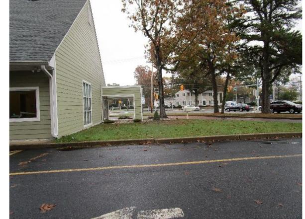
Parking spaces in the parking lot can be converted to porous pavement to capture and infiltrate stormwater runoff from the parking lot. A rain garden can be installed in the turfgrass area southeast of the building to capture, treat, and infiltrate stormwater runoff from the roof. A preliminary soil assessment suggests that the soils have suitable drainage characteristics for green infrastructure.
