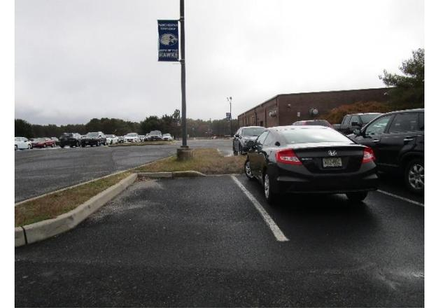
A section of parking spaces can be converted to porous pavement to capture and infiltrate stormwater runoff from the parking lot. Rain gardens can be installed in various locations to capture, treat, and infiltrate stormwater runoff from the roof or parking lot. A preliminary soil assessment suggests that more soil testing would be required before determining the soil's suitability for green infrastructure.
