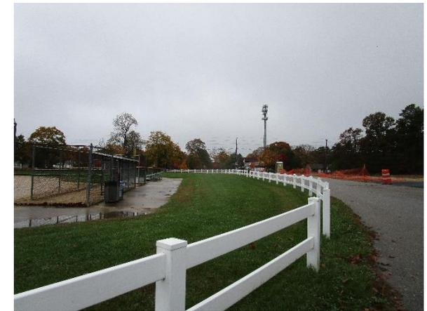
Parking spaces in the parking lot to the west of the baseball field can be converted to porous pavement to capture and infiltrate stormwater runoff from the asphalt. A rain garden can be installed in the turfgrass area near the dugout to capture, treat, and infiltrate stormwater runoff from the road. A preliminary soil assessment suggests that the soils have suitable drainage characteristics for green infrastructure.
